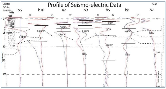
Figure 3. Seismoelectric (EKS) profile (west to east)
