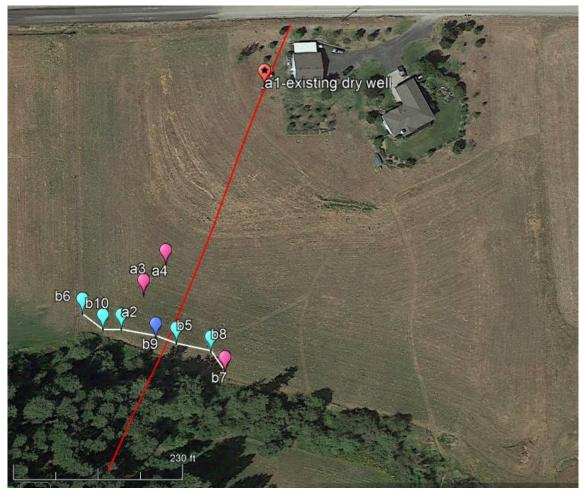
**Figure 2. Aerial photo courtesy Google Earth** Resistivity imaging profile (red), EKS profile of sites (white)
